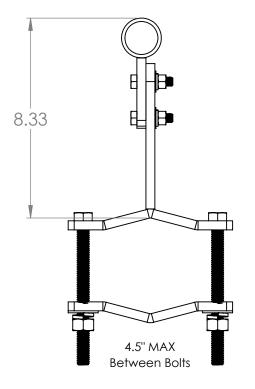
Will mount on tower legs from 1.5" to 4.5" dia. Reversing the outer clamp allows it to be attached to angle iron tower legs.
